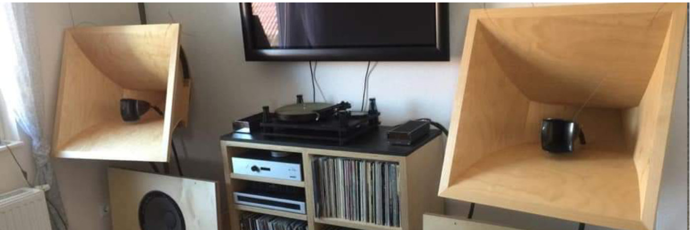
HT9-8060 "white" integrated into "flying" WE15a horn. Crossover 0.9khz, DSP
