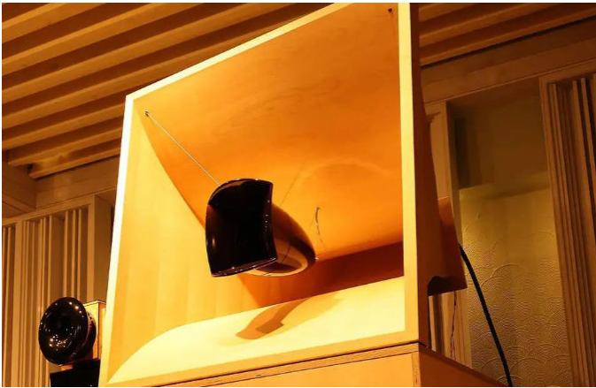
HT16-7040 "deep crimson purple" integrated into WE66 horn. Crossover 1.6khz, DSP
