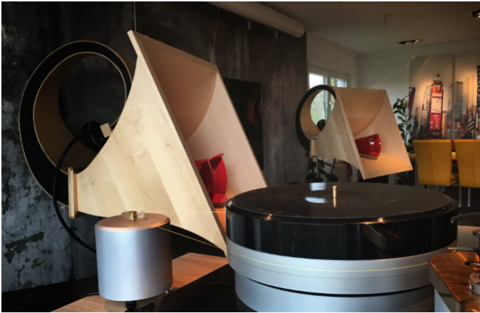
HT16-7040 "blood red" integrated into WE66 horn. Crossover 1.6khz, DSP
