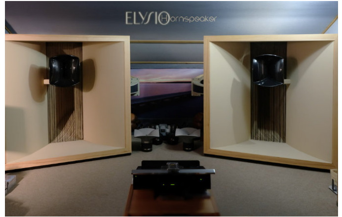
HT9-8060 "black" integrated into WE15a horn. Crossover 0.9khz, DSP
